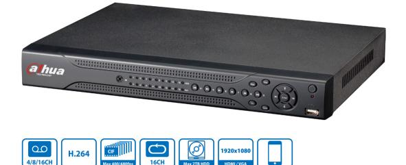
DH-DVR0404LE-A: 4 channel video inputs and 4 channel audio inputs. The 1st video channel can support max D1(4CIF) realtime recording and other channels can support CIF realtime recording. It can support VGA, HDMI and USB2.0.
